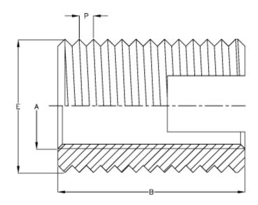
Female thread A = M3,5Length B = 6Male thread E = 5.0Min hole depth blind hole = 8Recommended bore diameter (hard mat.) = 4.6 to 4.7Recommended bore diameter (soft mat.) = 4.5 to 4.6Thread pitch P = 1.00Type  $= 303 \ 0 \ 035...$
